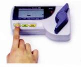
Press the "SELECT" button and repeat until the Selection Indicator of the sample you wish to test appears at the bottom of the display.
