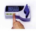
First,confirm that the figures "8 TIMES 88.8%" and several other marks appear when the "POWER" button is pressed with your finger. Should the figures not appear ,or any mark,the batteries are exhausted. Replace all of the batteries with new ones, according to the diagram illustrated in the battery chamber.
