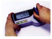
A Rotate the Crushing Handle counterclockwise, and fully insert the Sampling Tray into the Testing Chamber. Fully rotate the Crushing Handle until stop is reached, so that the sample may be well crushed. Press the "POWER" button, the most reliable moisture content is then displayed to be read directly without using any conversion tables.
